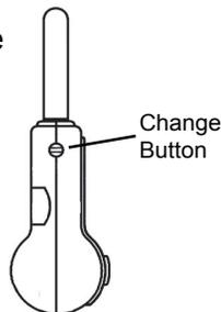
A new combination can be reset in the future by setting the dials to the opening shackle combination at that time prior to going to step #2
